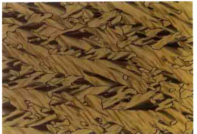
Figure 7. The parquet texture of the S_C^* phase in the homogeneous alignment cell with 2\mu\text{m} thickness obtained for (R,S)P9PBNP under crossed polarizing microscopy at 111.6^\circ\text{C} (magnification \times 150 ).
